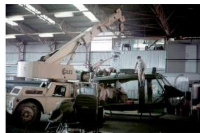
This is an interesting shot taken in early days with a Bravo model in deep repair; really, that's a fairly standard level of disassembly for the major 'D' servicing conducted by 9SQN – note the innovative use of ammunition boxes and sand bags as trestles.
